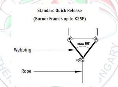
The maximum angle between webbing arms is limited to 60 or 90 degrees for preventing overstressing of the burner frame. For 60 degrees the lengths of the webbing arms are to be at least the same as the distance between their attachment points - envelope karabiners or attachment lugs.
